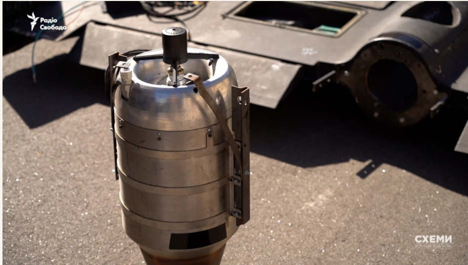
Plate 4. Exposed turbojet assembly shown in the examination; no independent performance test is presented. Schemes / Radio Svoboda, 19 September 2026; capture date unstated. [2]
